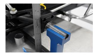
10. The last step in the process is to recheck the toe setting. We recommend to run no toe in or toe out. Lift the front of the car out of the blocks and set it back in to see if there is any drag on alignment blocks.
