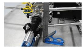
6. The next step in the process is to square the rear axle in the car. Using two squares and a ruler, measure from the back of the rear axle to the back of the rear cross tube, this measurement should be 5". Take this measurement as far out on the axle (on the left and right sides) as possible and adjust the rear radius rods by turning the top and bottom the same amount so you don't lose your bird cage timing.
