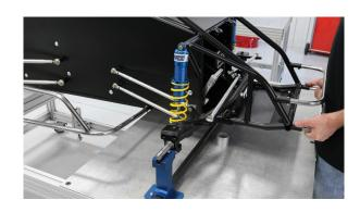
Adjust your tie rods so that the pitman arms on the steering shaft are in the 11 and 1 position and spindle bolts come in and out of blocks without dragging.
