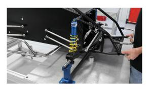
3. Once the car is down in the blocks, the next step is to set the side-to-side location of the axles. The left-to-right placement of the rear axle is determined by the location of the left rear bearing carrier. Place the inside edge of the carrier flush with the inside edge of the main rail of the chassis.
