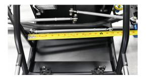
8. Once the rear axle has been squared in the car, we can use it to set the front axle. Simply measure from alignment bar to alignment bar on both sides of the car to get the center-to-center measurement of the axles.
