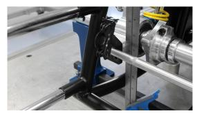
**4.** After axle placement, the bearing carriers need to be timed. Adjust LR Birdcage timing by using a square and adjusting the LR radius rods. Adjust the rods so that the square is flush against the panhard bracket.
