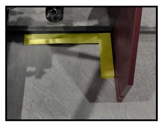
10. Once the toe is set measure the front alignment rod to the rear alignment rod on both sides to check the wheelbase. Adjust the right and left front tie rods to set the wheelbase to the proper measurement. (Make sure to keep the toe square as the wheelbase is adjusted.)
