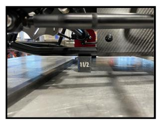
3. Install the Ultimate QM alignment plates in their correct positions and slide in the alignment bars. (If the rear plates will not sit flat you may need to remove the key from one of the rear hubs.)
